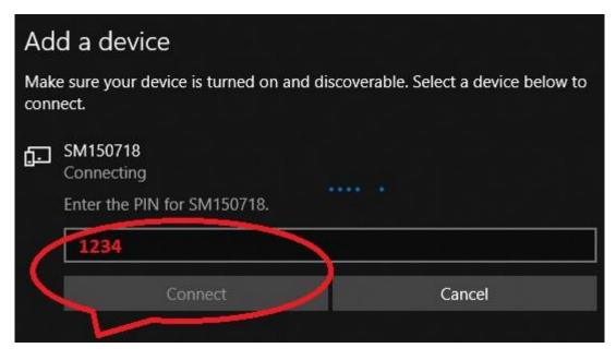
5. In ADD A DEVICE CONNECT page enter the connection PIN (normally 1234)
