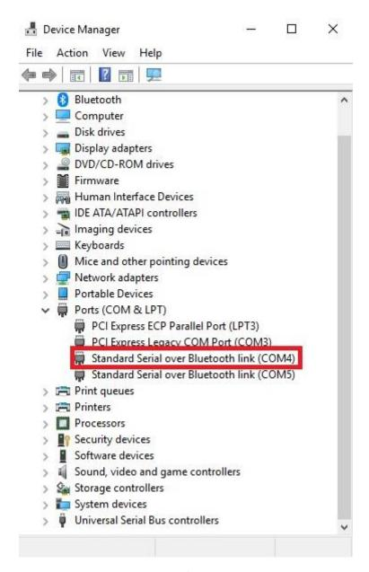
In DEVICE MANAGER the allocated Input/Output COM port number will be shown
